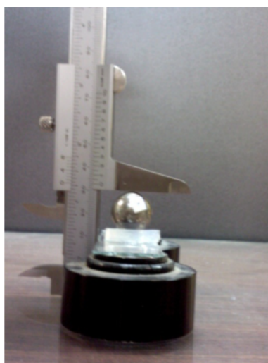
Fig 1. Indentation test set up for young's modulus measurement
